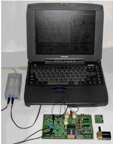
Playing around with Ohm's Law is fun because each is given some activity boards on which they can vary values of resistance; there are both a volt meter and an ammeter which can be used and they can do problems like predict current flow through a circuit. Different values of resistors are mounted on plugs on the board and there is a matrix with symbols so that it
